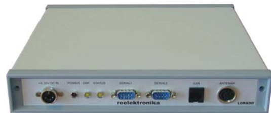
Figure 2 – ETRAN receiver specially developed for the measurement campaign.
