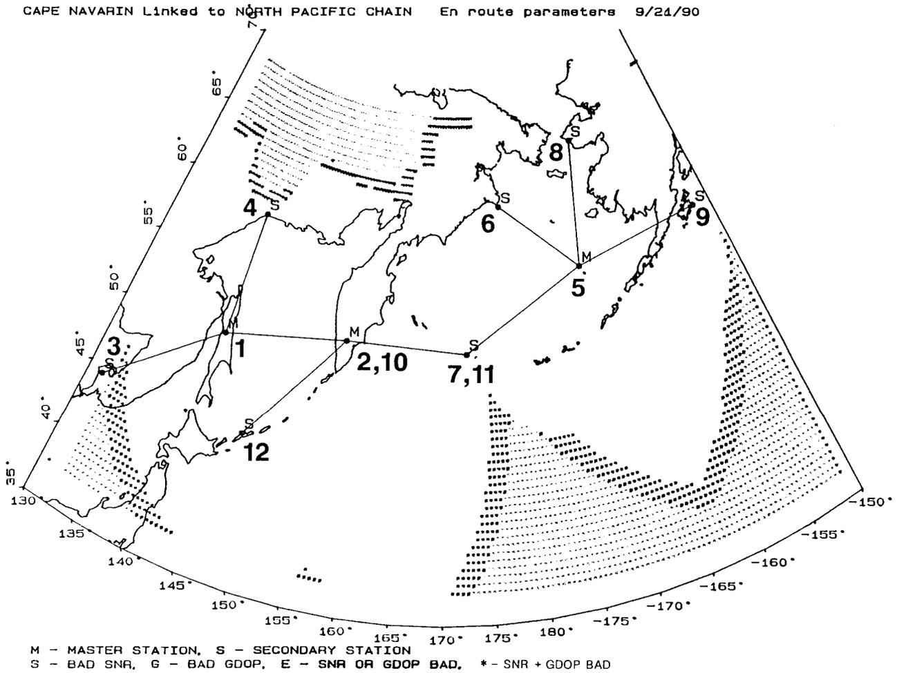
Plot #5 shows another possible connection for the Cape Navarin transmitter, linking it into the proposed Bering Sea Chain. The baseline is about 872 nautical miles. A good saltwater path is present. Although this new station adds some more coverage, its real advantage is to add a good geometrical triad traveling from Alaska to the Eastern area of Soviet Union across the Kamchatka Peninsula.
