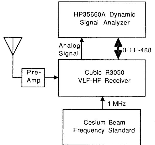
Figure 12. Spectral Analysis System for 0.01-30 MHz.
