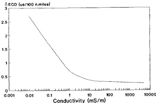
Fig. 3 Rate of change of ECD versus path conductivity. (After Sherman [10]).
