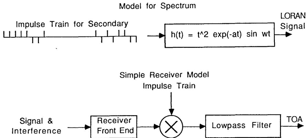
Figure 1. Model of for Calculation of LORAN Spectrum and Analysis of Interference.
