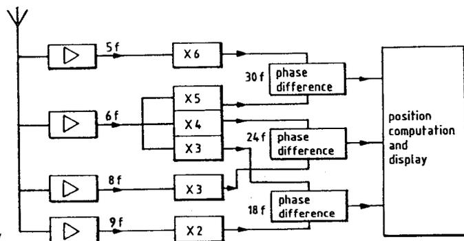
At first sight, therefore, Loran-C and the DNS appear to be fundamentally different systems. Loran employs broad-band pulses while the DNS uses a narrow-band CW technique. But the essential similarity is that both are hyperbolic systems, operating in the 100 kHz band, in which fine time-difference measurements are made by the comparison of carrier phase, the cycles being identified by means of a pulsed transmission. And in matters of groundwave propagation the differences are trivial.
