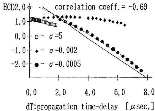
Fig. 5-2 Correlation of ECD and propagation time delay. (- linear, --- nonlinear)
