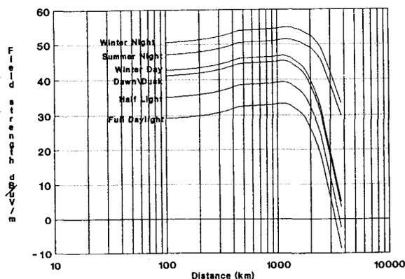
Fig. 7 99%ile skywave signal levels for various Decca Periods. Normalized for 1kW Radiator.
