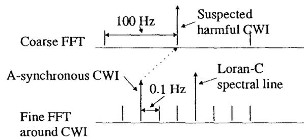
Fig. 17. Zooming in on an area with suspected harmful CWI.
