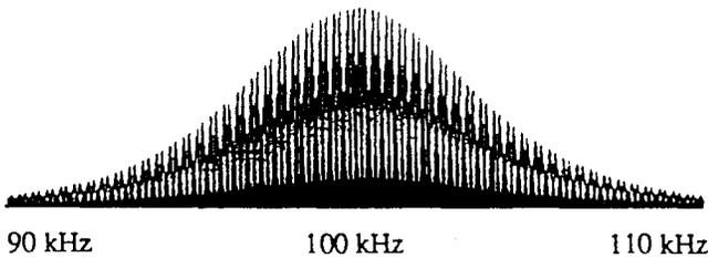
Fig. 9 Power spectrum of Loran-C transmission (After Beckmann [18]).
