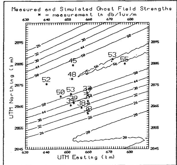
Figure 12. Brownsville Area Simulated and Measured Ghost Field Strengths
