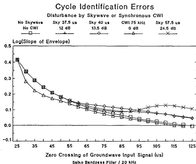
Fig. 6 Cycle identification error due to skywave or synchronous CWI.
