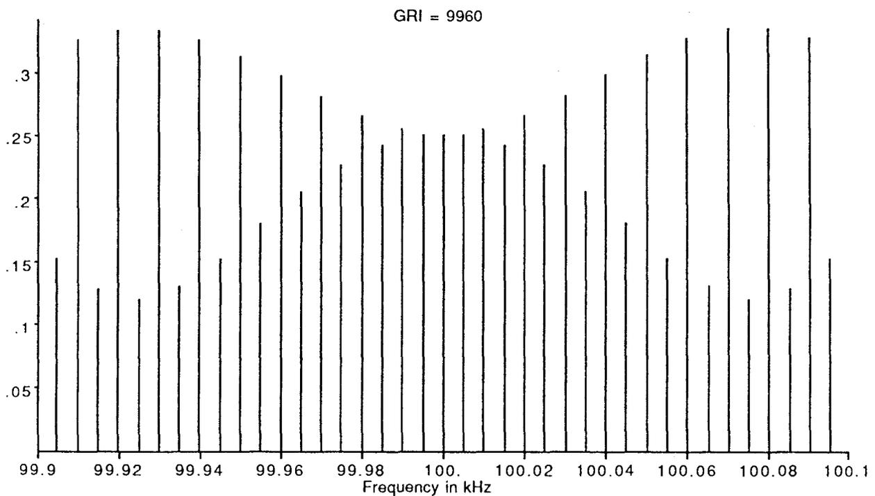
Figure 2. Plot of  $|X(w)|/16$  showing the spectral line structure in the region of 100kHz.
