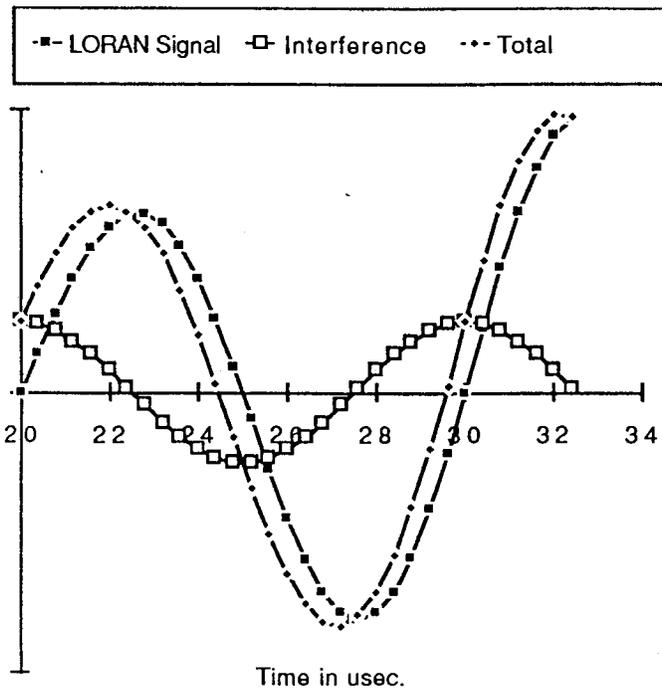
Figure 3. Shift in zero crossing due to sinusoidal interference.
