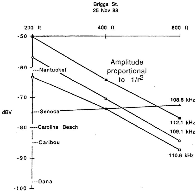
Figure 9. Power Line Carrier Strength vs. Distance and Relative to LORAN Signal Strength.
