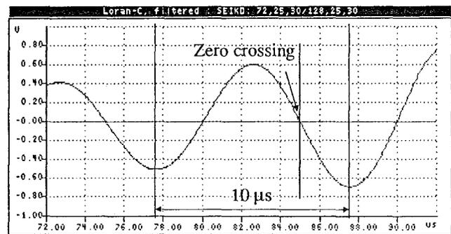
Fig. 4. Loran-C pulse with zero crossing for tracking.
