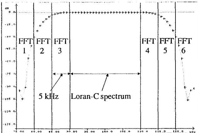
Fig. 18. Breaking up the CWI spectrum into segments.
