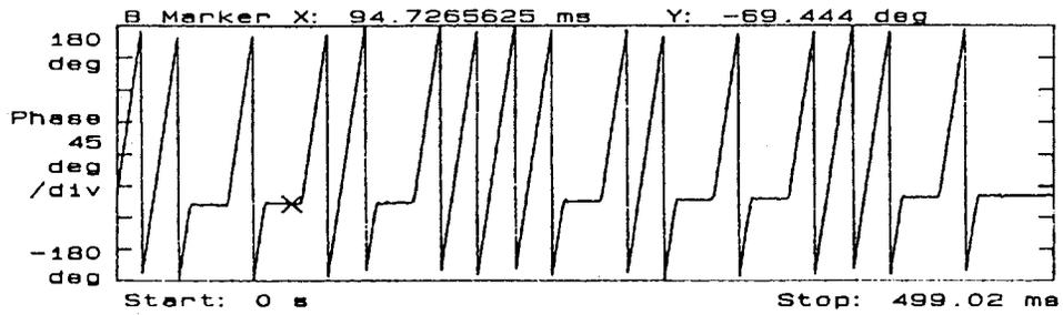
Figure 10. Frequency Shift Keyed (FSK) Signal from Driver, VA.
