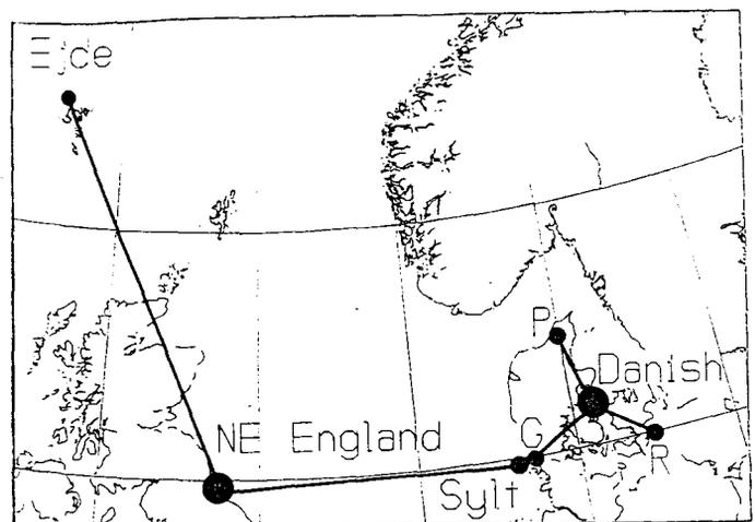
Fig. 10 Off the Danish west coast Loran-C ASFs are negligible since, though paths are long, they lie almost entirely over sea-water. Decca Navigator ASFs are substantial because the master signal must cross the land-mass of Jutland.
