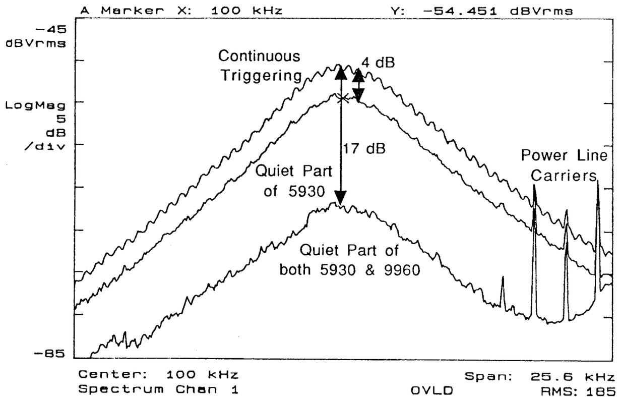
Figure 7. Effect of triggering in quiet part of GRI
