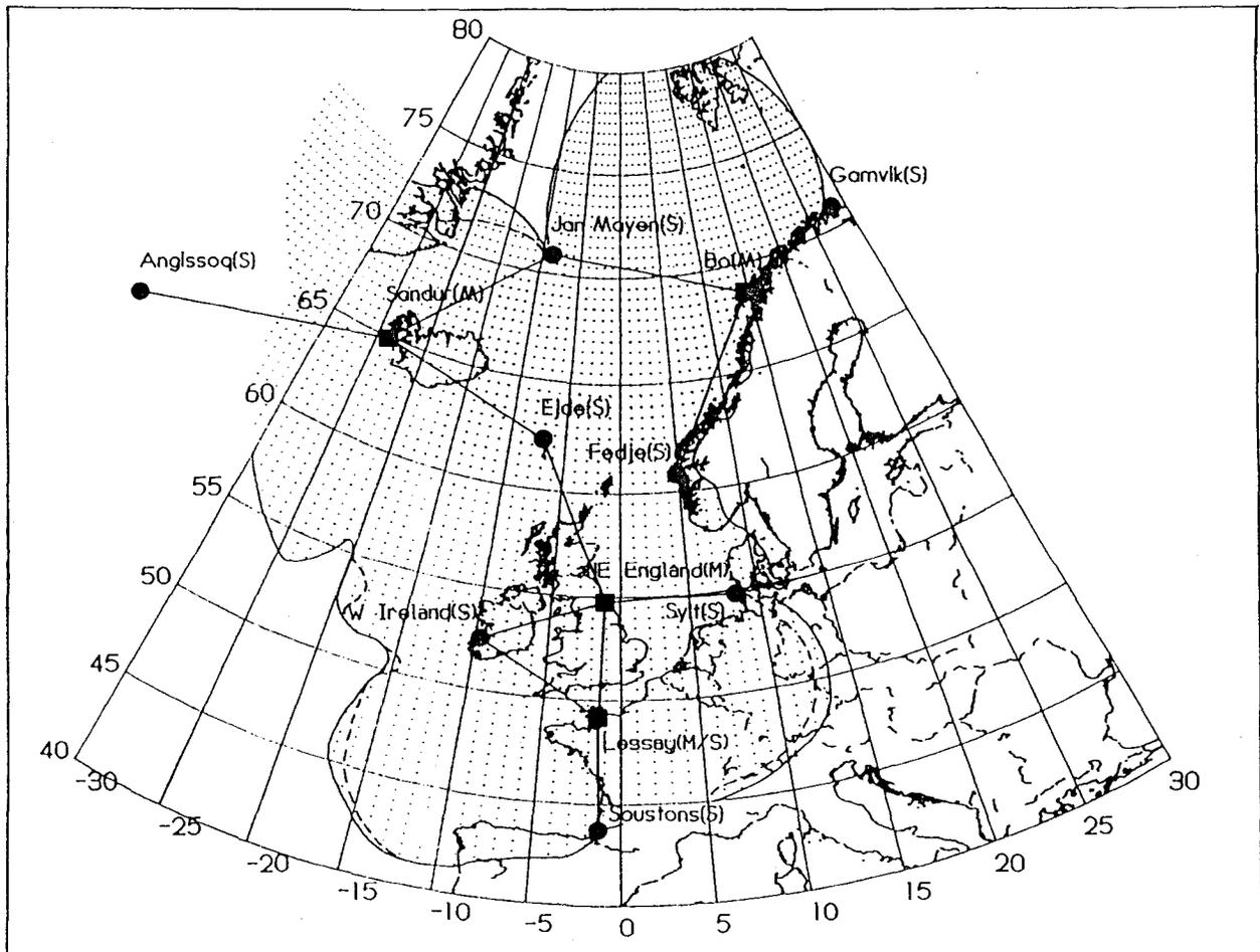
Fig. 4 Coverage of proposed North-West European Loran-C system [12]. Within the solid contour the absolute accuracy is predicted to be 463m (95% confidence).
