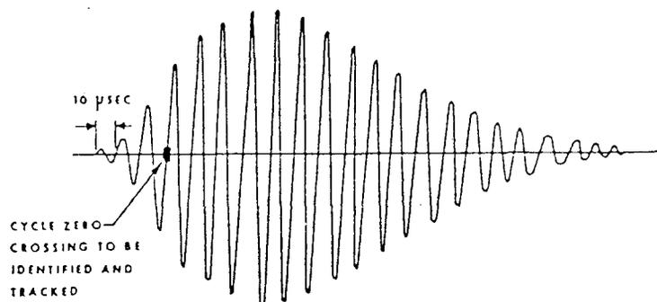
Figure 5. 100-kHz LORAN-C pulse. A receiver locks onto the third cycle crossover [6].
