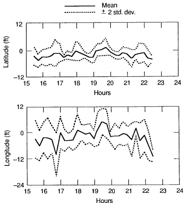
**Figure 7** Differences in position between LONARS I and LONARS II systems on the U.S.S. Range Sentinel tracking the same signal on day 120, April 30, 1990.
