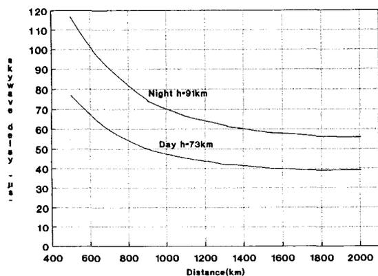
Fig. 6 Skywave delay from Loran-C rate tables [11]
