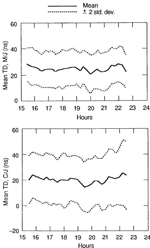
**Figure 6** Differences in TDs between LONARS I and LONARS II systems on the U.S.S. Range Sentinel tracking the same signal on day 120, April 30, 1990.
