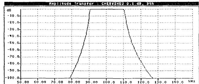
Fig. 4. A filter with steep slopes used for removing CWI.
