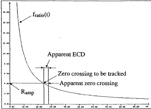
Fig. 10. Calculation of the apparent ECD.
