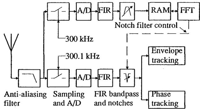
Fig. 19. Receiver with tuneable bandpass filter and FFT.
