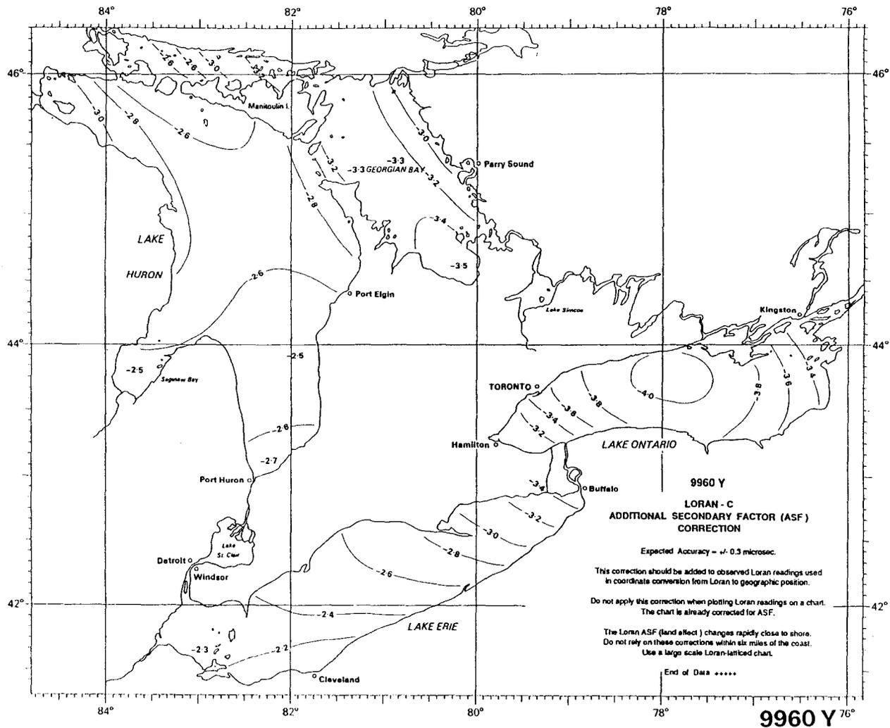
Fig. 8 Plots of additional secondary factors of time differences determined by the Canadian Hydrographic Service by computer modelling and survey [15].
