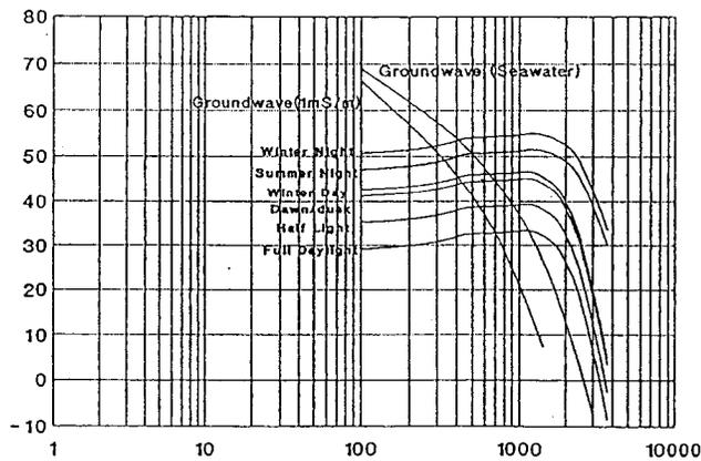
Fig. 2 Groundwave and skywave signal level as function of distance with time as parameter. Ground conductivity is 1 mS/m, fieldstrength in dB $\mu$ V/m, radiated power = 1 kW [1].
