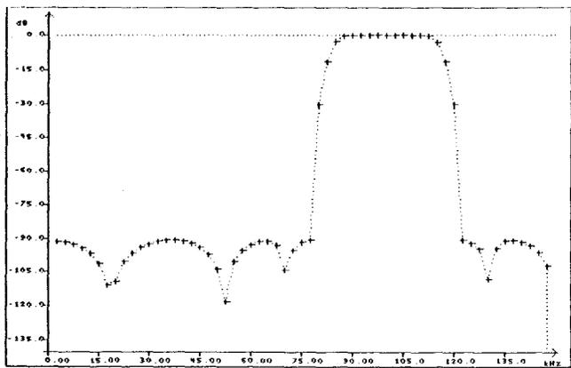
Fig. 12. FIR filter useful for bandpass sampling.
