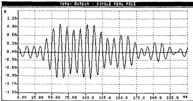
Fig. 2. Envelope distortion caused by CWI.
