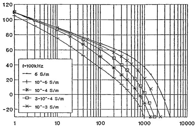
Fig. 8 Groundwave propagation for different values of conductivity [1]. Field-strength in  $\text{dB}\mu\text{V}/\text{m}$ , radiated power is 1 kW.
