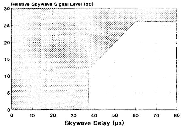
Fig. 5 IEC Skywave specifications [9]. Combinations of relative signal level and delay outside the clear area are out of limits.
