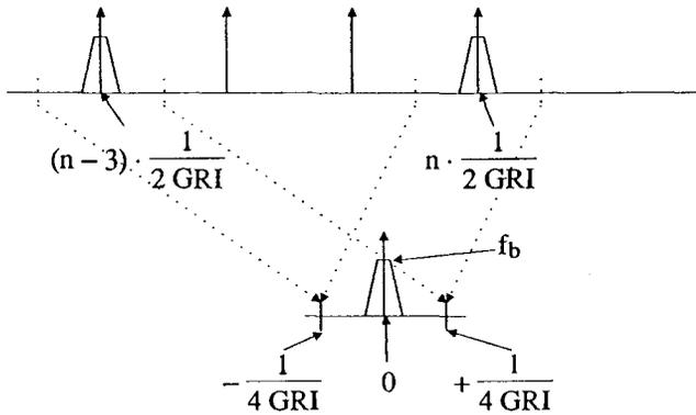
Fig. 2. Spectrum fold-back due to sampling pattern.
