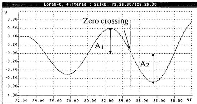
Fig. 7. Cycle Identification in linear receivers.
