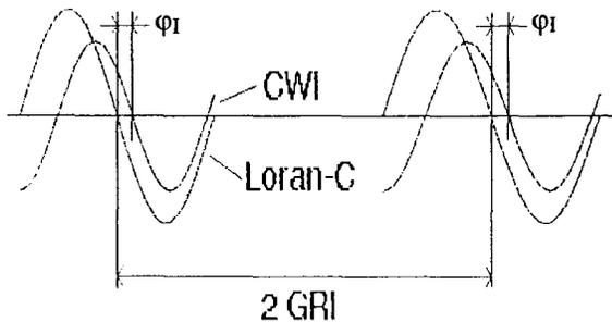
Fig. 3. Phase relation of synchronous CWI and Loran-C.
