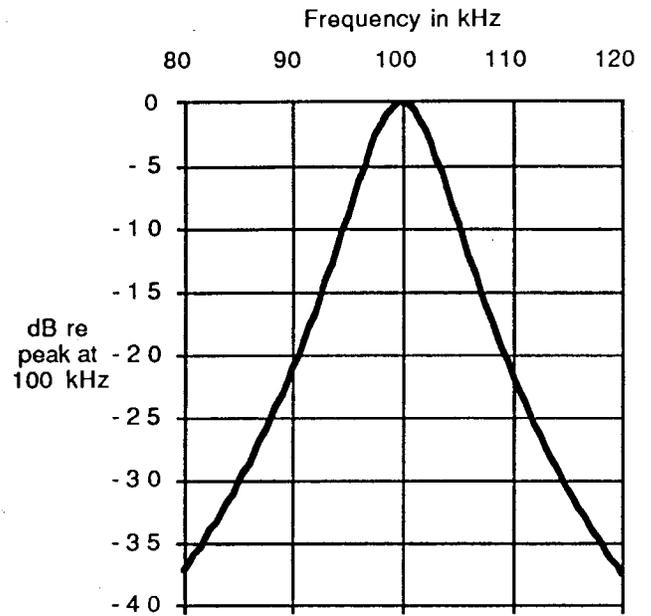
Figure 4. Coarse spectrum of LORAN.
