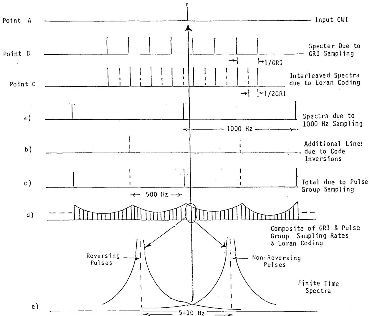
FIGURE 1 DEVELOPMENT OF FREQUENCY SPECTRA AS SEEN BY THE LORAN -C DETECTOR
