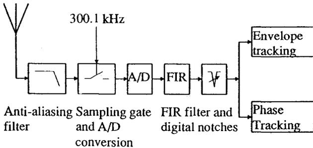
Fig. 13. Receiver with FIR filter and digital notches.
