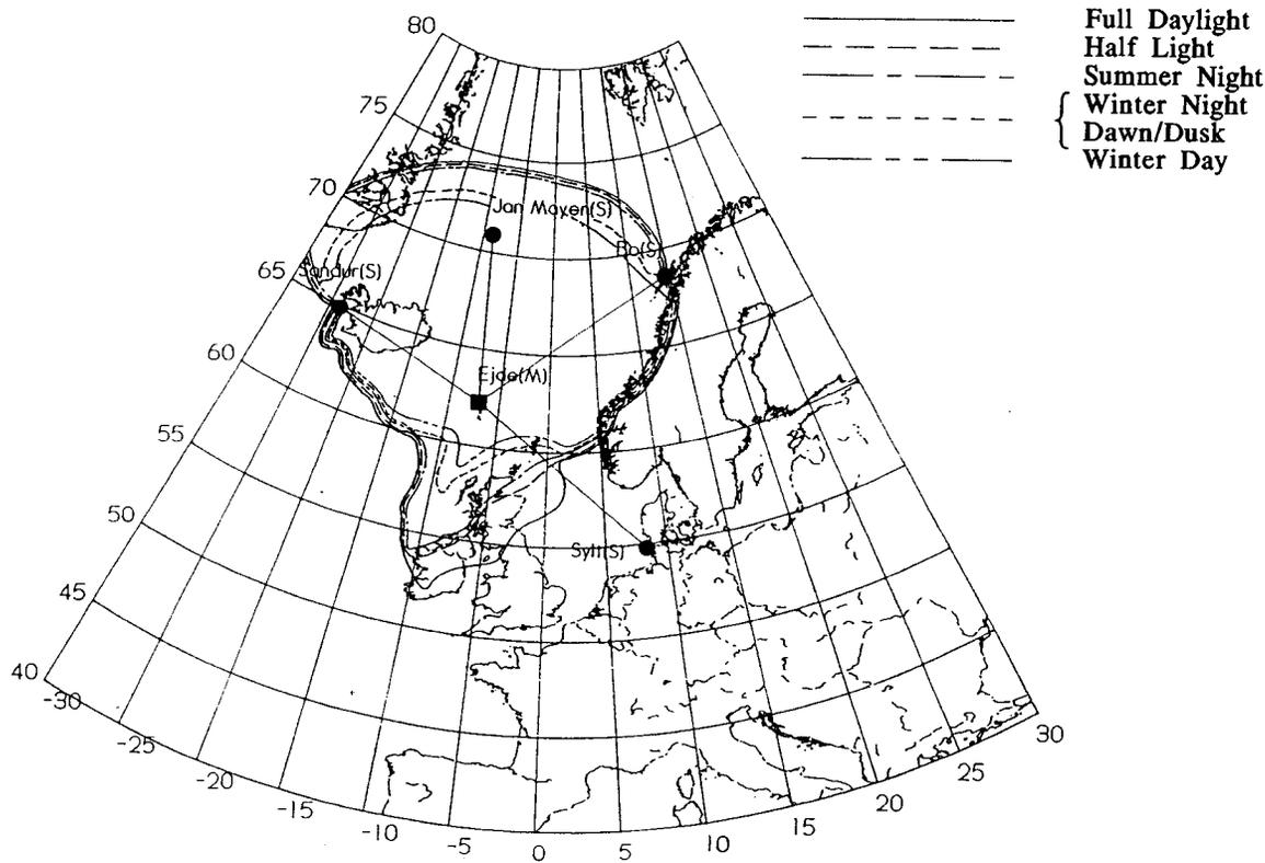
Fig. 8 Norwegian Sea chain coverage for various times and seasons showing skywave coverage limits.
