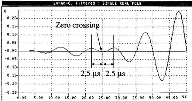
Fig. 6. Combined signal in a traditional CI circuit.
