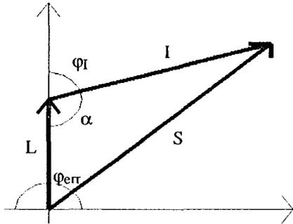
Fig. 11. Phasor diagram used for analysis.
