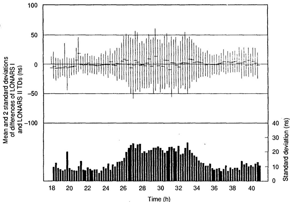
Figure 5 Differences in TDs between LONARS I and LONARS II systems at Cape Canaveral tracking the same signal.
