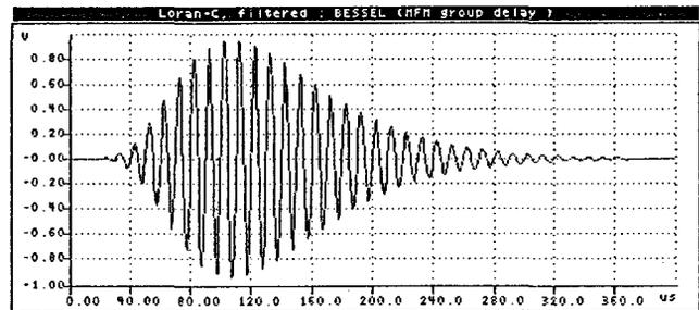
Fig. 9. Loran-C pulse filtered with the filter of fig. 7.
