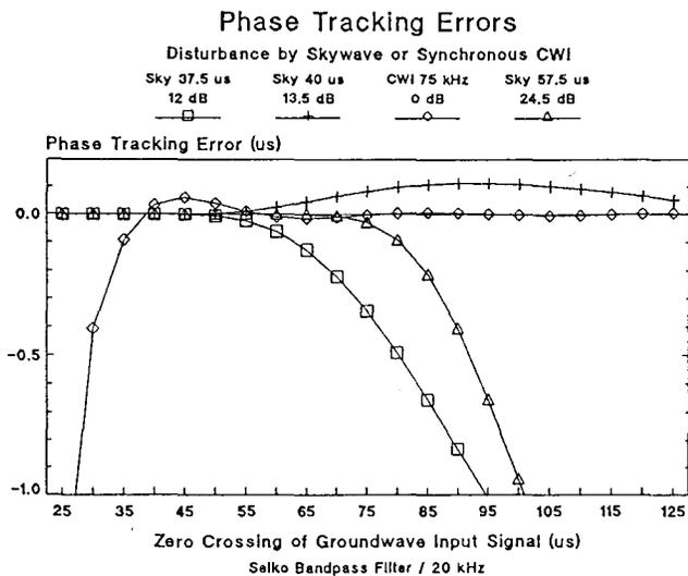
Fig. 5 Phase tracking error due to skywave or synchronous CWI.
