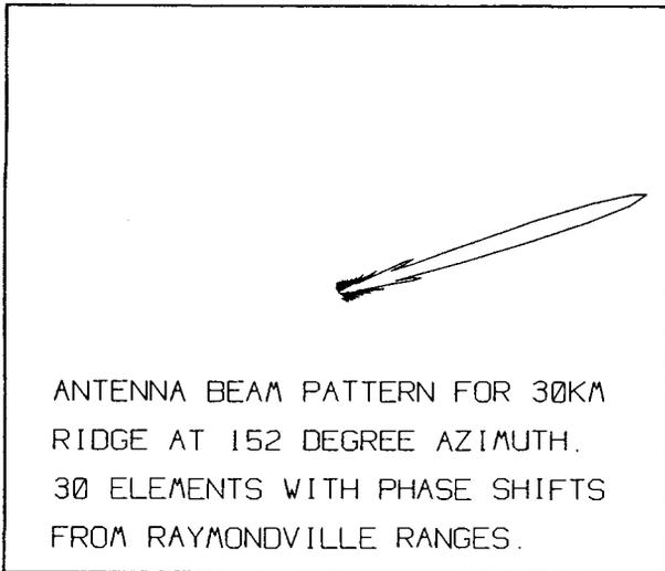
Figure 10. Antenna Beam Pattern
