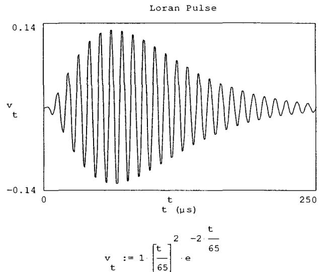
Figure 1. Loran Pulse
