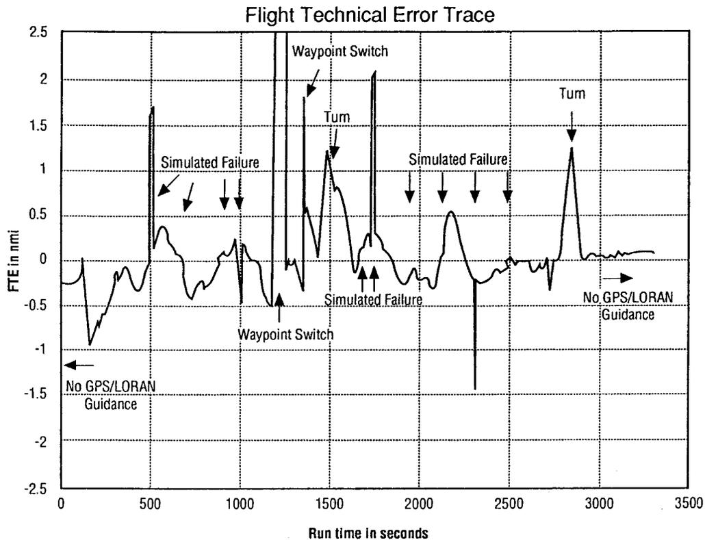
Figure 4 Flight Technical Error for Flight Two
