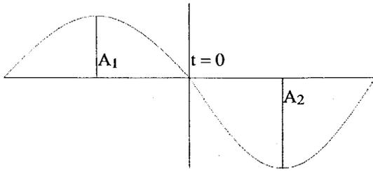
Fig. 8. Definition of a Loran-C signal for analysis.
