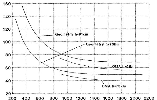
Fig. 1 Variation of skywave delay ( $\mu$ s) with distance for different effective ionospheric heights [1]. The geometry data are calculated, while the DMA data are derived from USCG tables.
