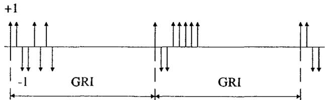
Fig. 1. Sampling pattern for Master station.
