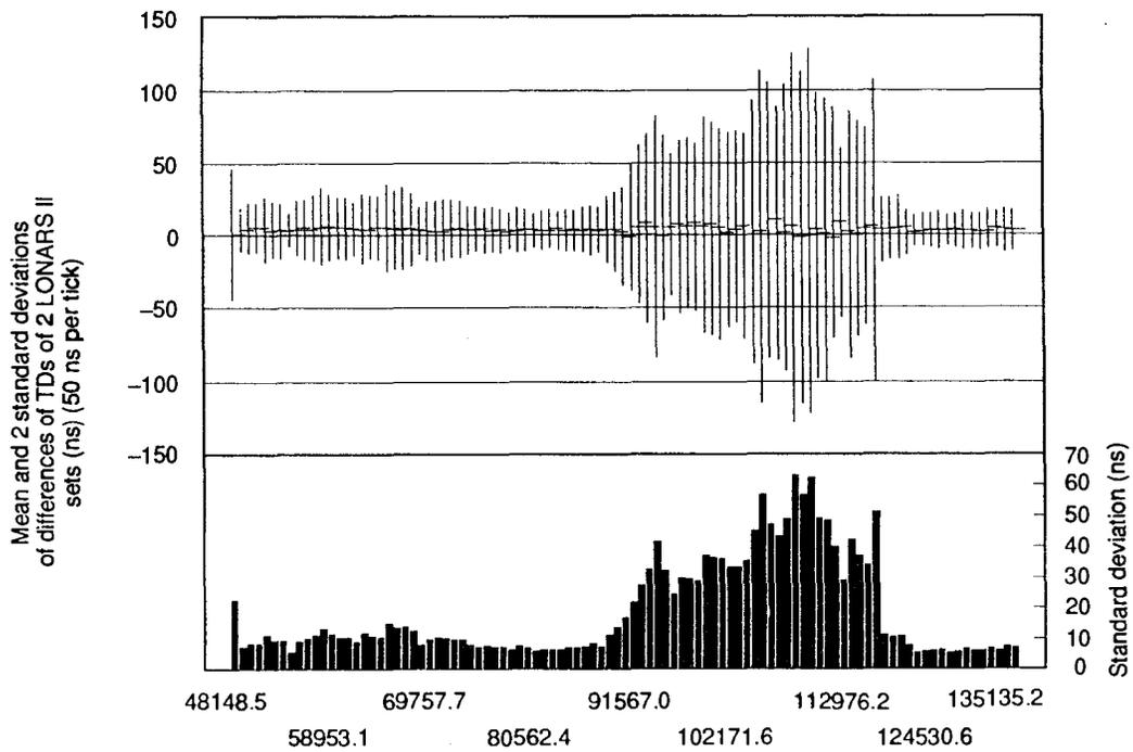
Figure 4 Differences in TDs between two LONARS II systems at APL tracking the same signal.
