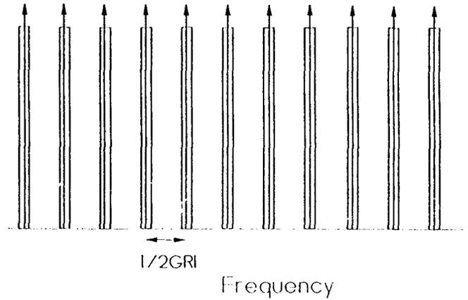
Fig. 10 Idealised comb filter transfer function.
