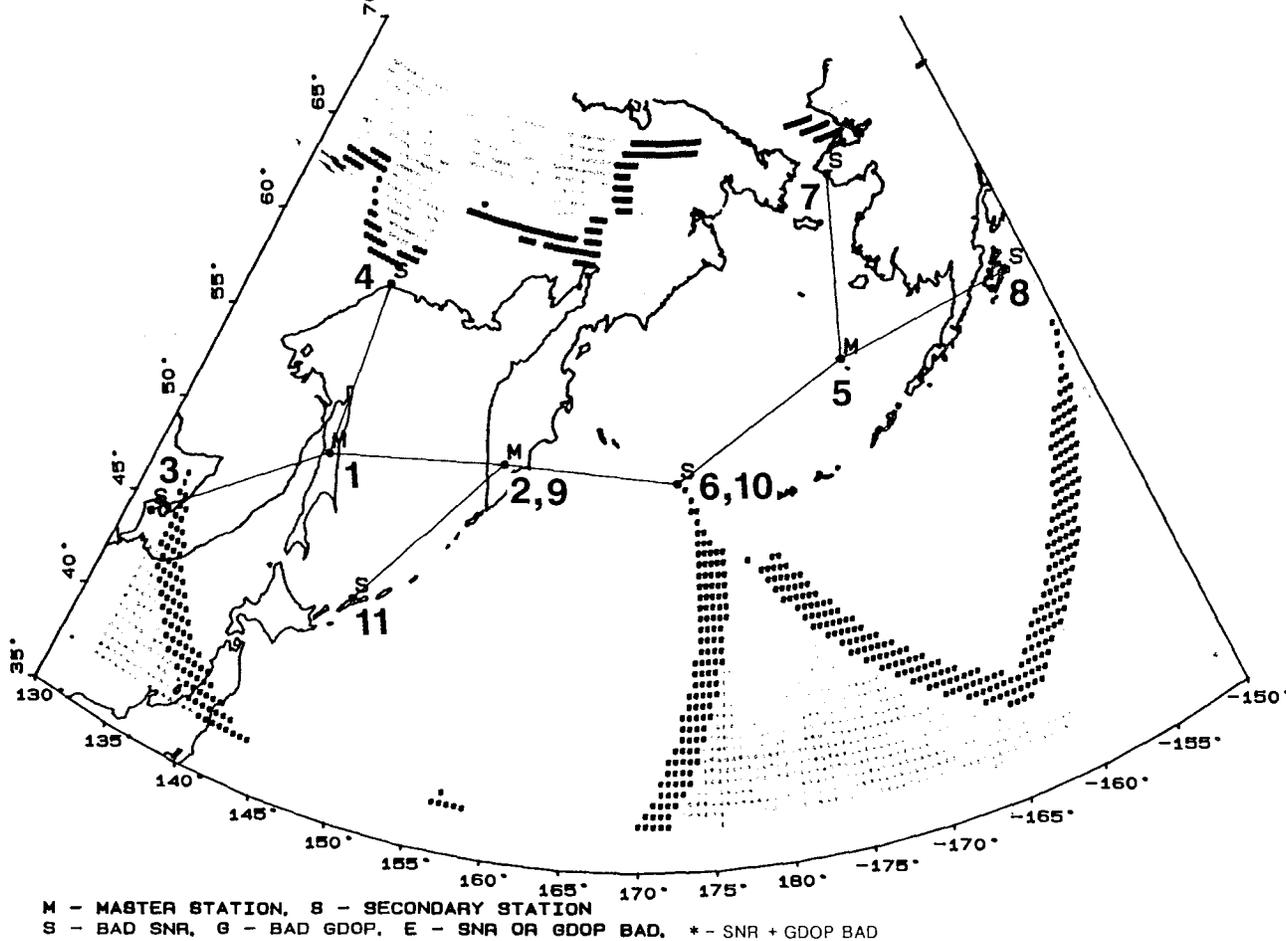
Plot #4 shows the addition of a transmitter at Cape Navarin linked into the North Pacific Chain, which effects an increase of coverage in the Northern Bering Strait area. The addition of the triad makes traveling north through the Bering Strait, Soviet Union, and Alaska towards the Arctic circle more accessible.
