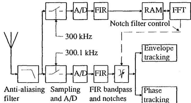
Fig. 16. Receiver architecture for zoom-in FFT.
