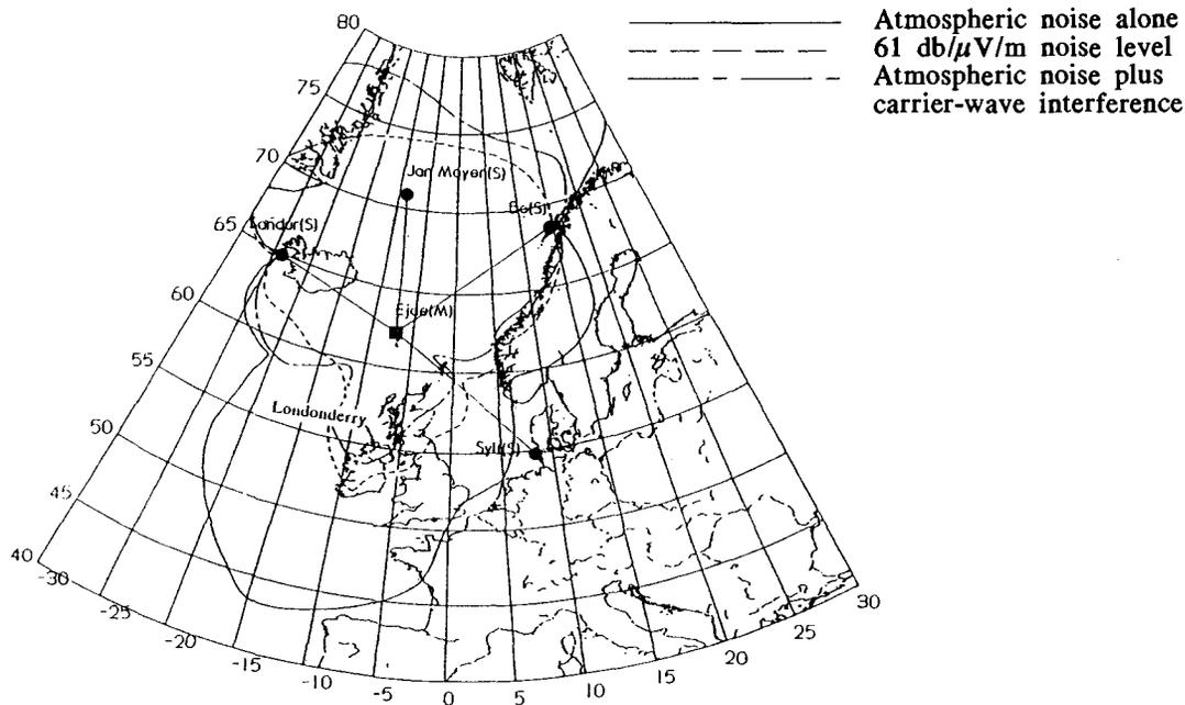
Fig. 12 Norwegian Sea Chain showing various coverage limits.
