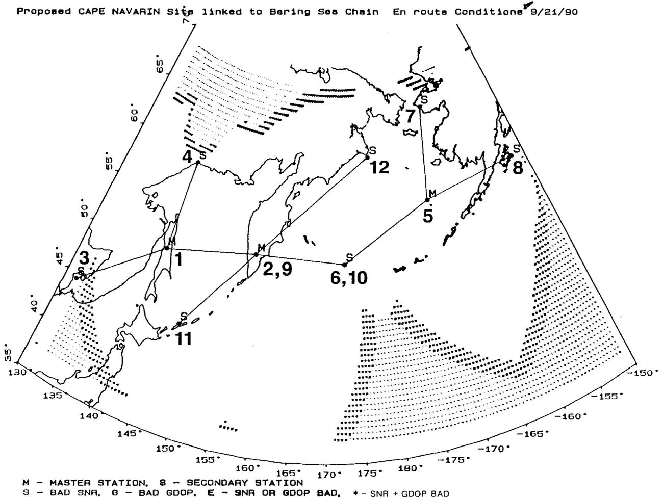
Plot #6 indicates the ultimate in coverage and triad tracking. With the proposed Cape Navarin transmitter linked to both the North Pacific and Bering Sea Chains, many combinations of triads exist. This newly expanded network makes traversing the North Pacific, whether by air or sea, a much safer venture.
