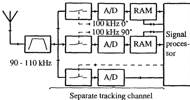
Fig. 15. An architecture useful for spectrum analysis.
