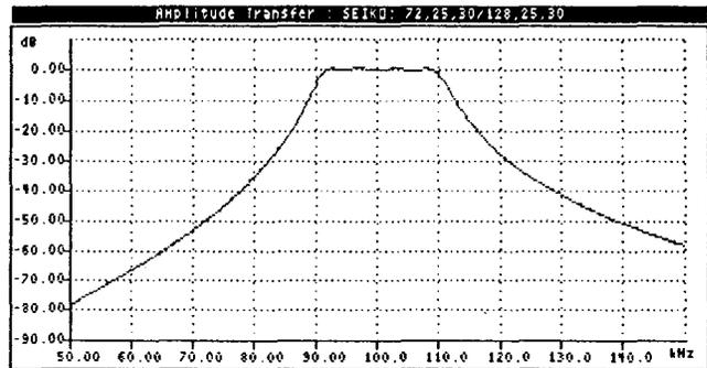
Fig. 14. Amplitude transfer function of SEIKO filter.
