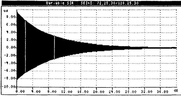
Fig. 15. Envelope shift as function of SIR - an example.
