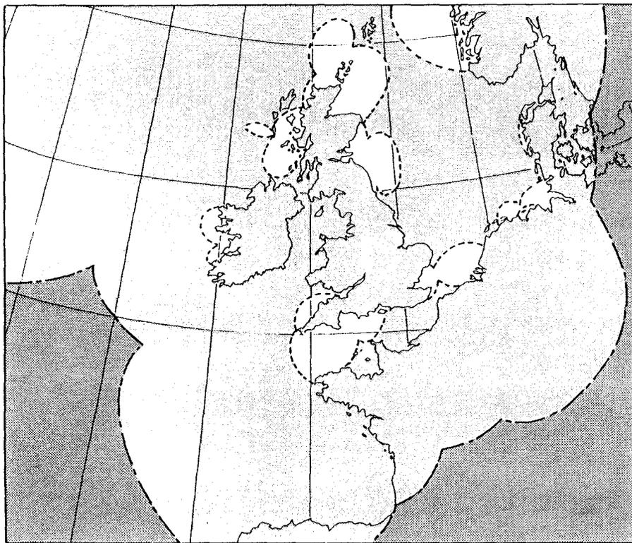
Fig. 6 Areas within which the Loran-C (— — —) and the Decca Navigator System (— — —) repeatabilities are better than 400m (95% confidence) at all times and seasons (DNS land coverage omitted) (after [2]).
