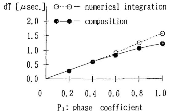
Fig.2-2 Relation between phase characteristic and propagation time-delay ( $n=0.5$ )
