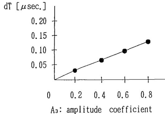
Fig.2-1 Relation between amplitude characteristic and propagation time-delay ( $m=0.5$ )
