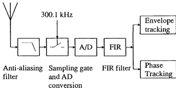
Fig. 10. Receiver with a FIR bandpass filter.
