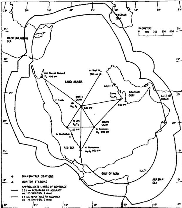
Figure 3. Saudi Arabia Loran-C Coverage
