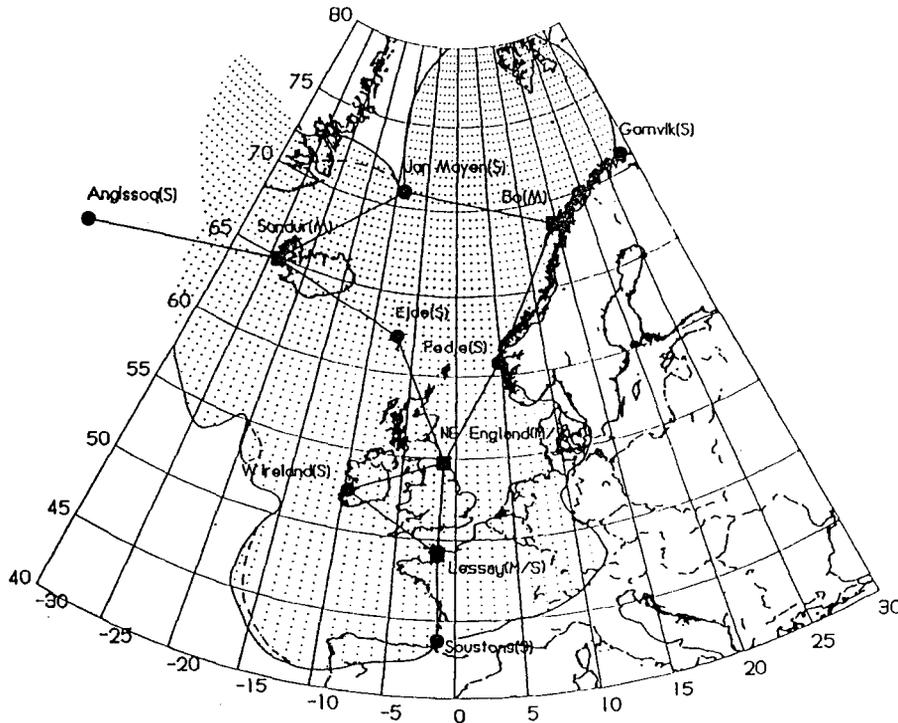
Fig. 2 Coverage of the proposed N.W. European Loran-C system. Within the solid contour the absolute accuracy is predicted to be 463m (95% confidence).
