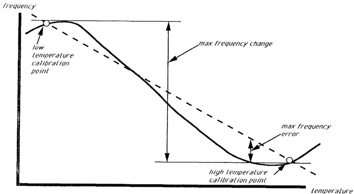
Figure 5 WORST CASE ERROR WITH STRAIGHT LINE PREDICTION
