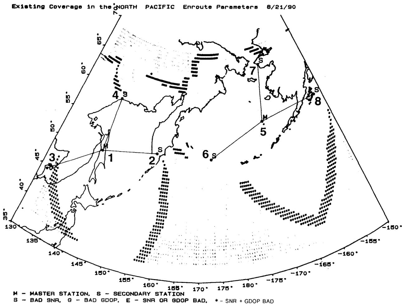
Plot #3 shows the proposed Bering Sea Chain, which links the Loran and Chayka Systems. It opens a large area of ocean coverage--from the 155 degree east meridian to the 170 degree meridian (West of the International Date Line)--by upgrading the low power Kurilsk Station (6 KW, similar to Station Okhotsk) to 300 KW. Kurilsk and North Pacific Chain's Attu are secondaries to the newly dual-rated master station Petropavlovsk.
