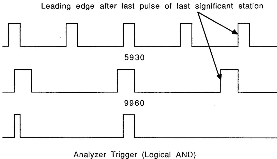
Figure 6. Timing diagram of circuit to trigger in quiet of both GRI's.
