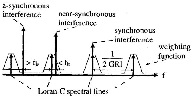
Fig. 14. Example of a weighting function.
