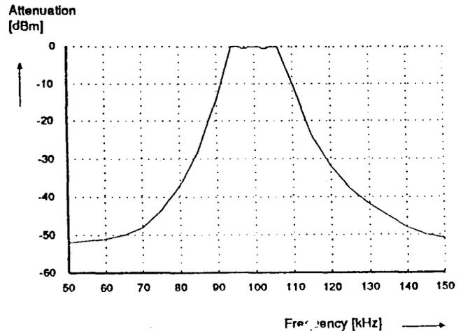
Fig. 11 Transfer function of the 'standard' bandpass filter (After Beckmann[18]).
