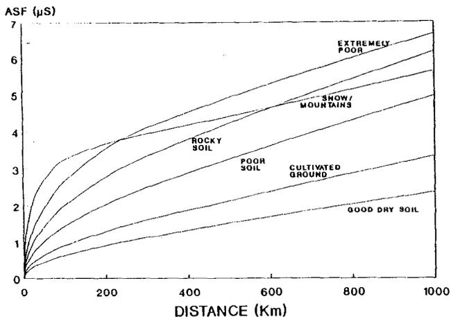
Fig. 7 Growth of additional secondary factor (due to propagation over land) with distance for various types of terrain (after Brunavs [14]).
