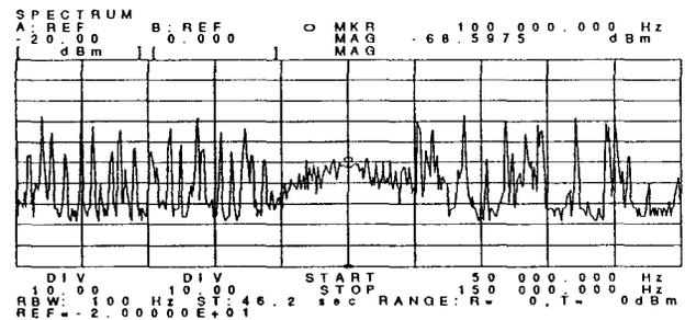
Fig. 3. European CWI spectrum from 50 to 150 kHz.
