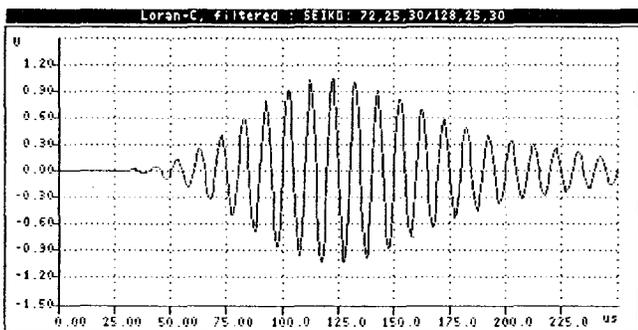
Fig. 13. Loran-C burst filtered with SEIKO filter.
