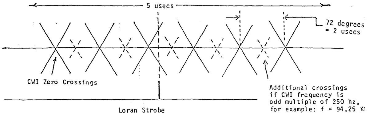
FIGURE 2 PHASE QUANTIZATION DUE TO SUBSYNCHRONOUS CWI OF 94.5 KHz FOR LORAN RATE 9940
