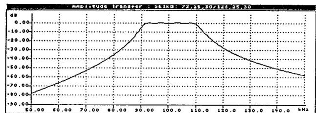
Fig. 3 Amplitude transfer function of 20 kHz wide simulated Seiko bandpass filter.
