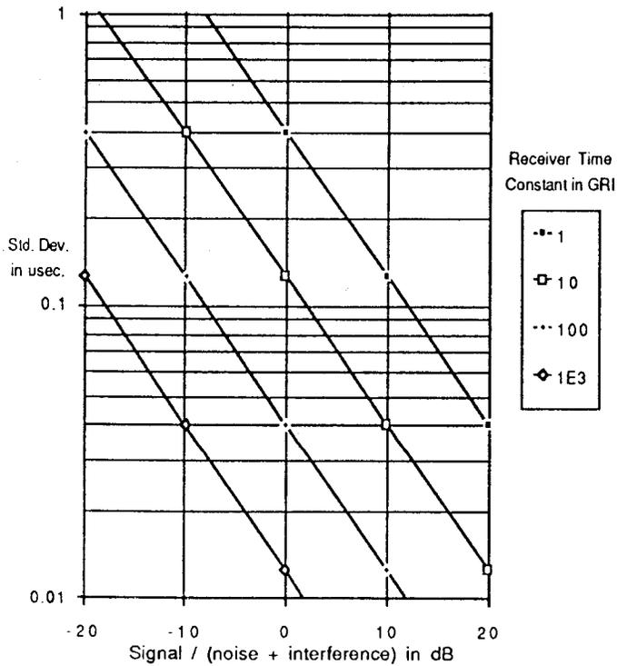
Figure 11. Phase noise vs. signal / (noise + interference).
