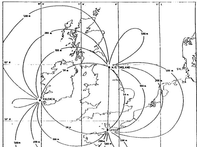
Fig. 3 Contours of repeatable accuracy (95% confidence) for a Loran-C triad consisting of a master station in N.E. England and secondary stations at Lessay, France and Valencia, Ireland (after Megapulse [3]).
