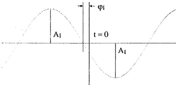
Fig. 9. Definition of a CWI signal for analysis.
