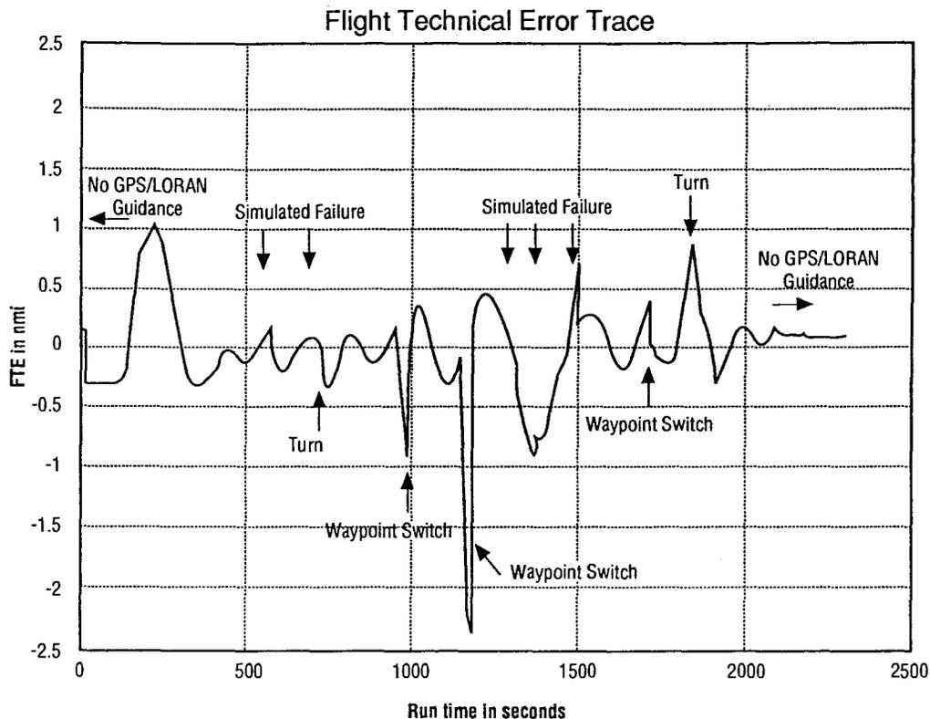
Figure 3 Flight Technical Error for Flight One
