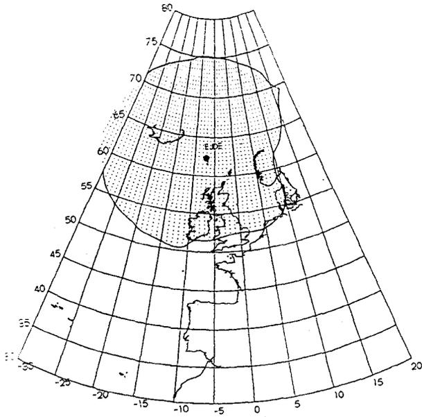
Fig. 1 Coverage of the Loran-C Transmitter at Ejde in the Faeroe Islands. Assuming a noise level of 61 dB  $\mu$ V/m
