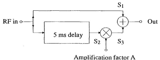
Fig. 5. Traditional Cycle Identification circuit.
