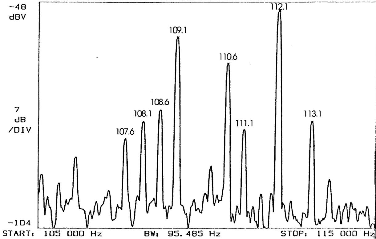
Figure 8. Typical Spectrum of Power Line Carriers.
