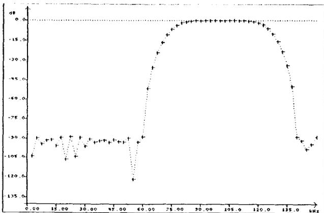
Fig. 11. A FIR bandpass filter with order 53.
