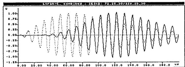
Fig. 4 Input (dotted line) and output (solid line) Loran-C signals of simulated Seiko bandpass filter.
