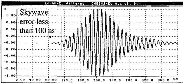
Fig. 5. Loran-C pulse filtered with the filter of fig. 4.
