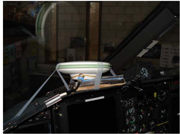
Figure 2. The antenna installation for the helicopter test
