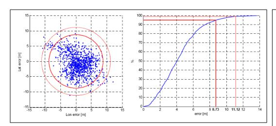
Resulting dLoran HEA positioning error with respect to DGPS:
