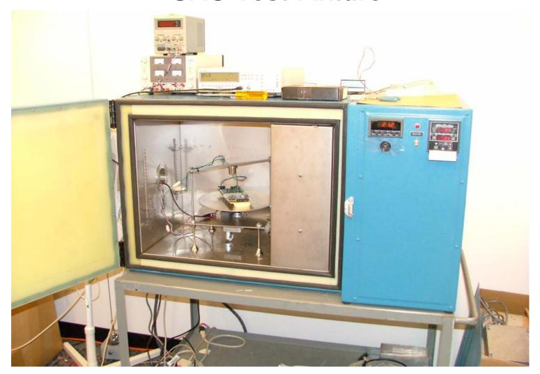
Rotation rates of 0 - 50 rpms Temperature range - 50° C to + 80° C
