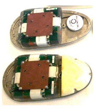
• Combined GPS/Loran antenna in ADF radome for flight trials
